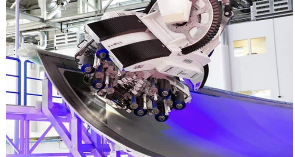
The MTorres automated fibre placement head at Airbus applying composite tape to an A350 wing cover tool
